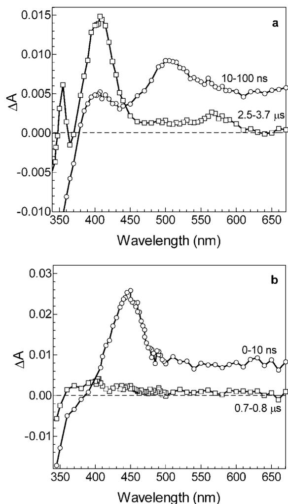
**Figure 2.** Transient absorption spectra recorded by 337-nm laser flash photolysis of deoxygenated MeCN solutions of (a) 4-dimethylaminobenzophenone (**1**; 0.1 mM) + phenol (0.8 mM); and (b) 4-dimethylaminoacetophenone (**15**; 0.1 mM) + 4MP (9.9 mM).
