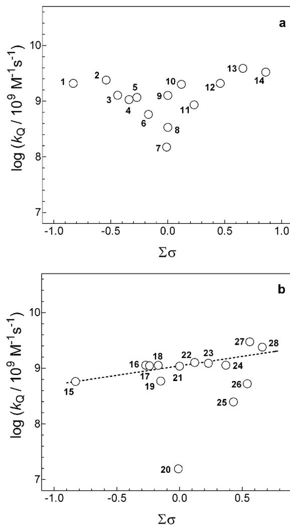
**Figure 3.** Plots of  $\log k_Q$  versus Hammett substituent constants ( $\Sigma\sigma$ ), for the quenching of substituted benzophenone (a) and acetophenone (b) triplets by 4MP in deoxygenated MeCN solution at 23°C.
