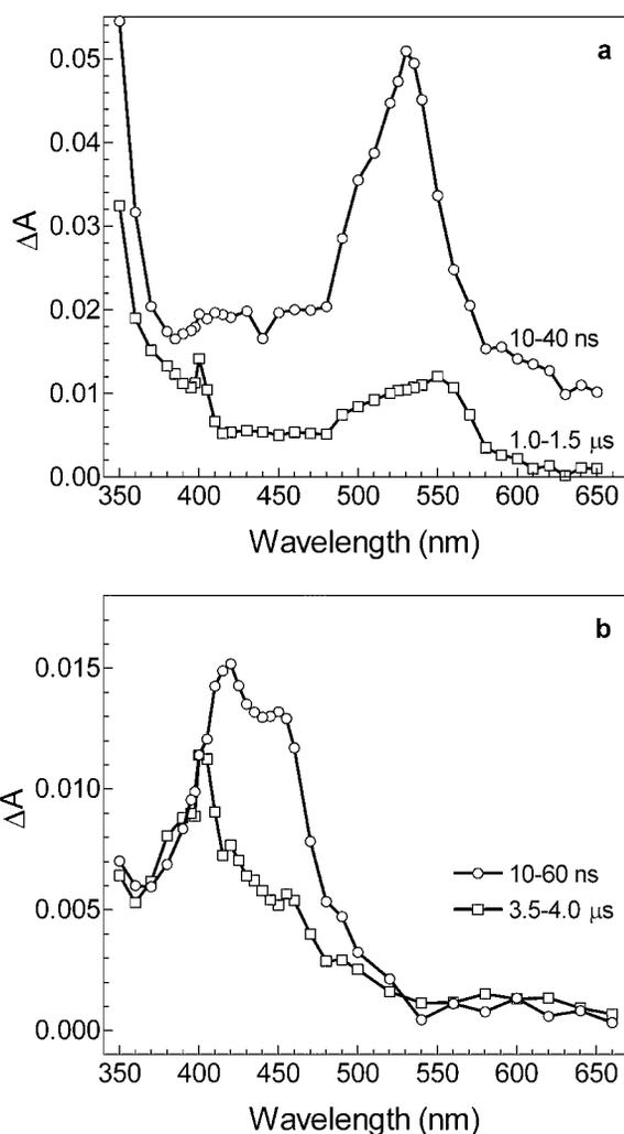
**Figure 1.** Transient absorption spectra recorded by 337-nm laser flash photolysis of deoxygenated solutions of (a) 4-bromobenzophenone (**11**; 3.8 mM) and (b) 4-trifluoromethylacetophenone (**26**; 68 mM) in MeCN in the presence of 4–6 mM 4MP.
