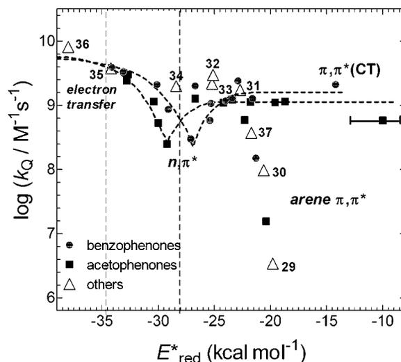
**Figure 5.** Plots of  $\log k_Q$  versus triplet state reduction potential ( $E_{\text{red}}^*$ ) for the quenching of 1–14 and 16–37 by 4MP in deoxygenated MeCN solution at 23°C. The shaded area between  $-28.1$  and  $-34.6$  kcal mol $^{-1}$  represents the range of uncertainty in the (thermodynamic) half-wave oxidation potential of 4MP.
